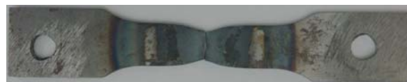
Fig.5 The tensile test specimen at the strain rate of 0.1s -1 and the temperature of 1123K
