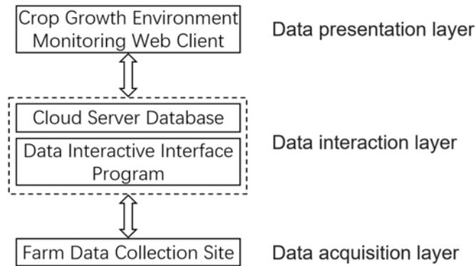
Fig.1 The research and design of intelligence environment monitoring and evaluating system frame diagram
