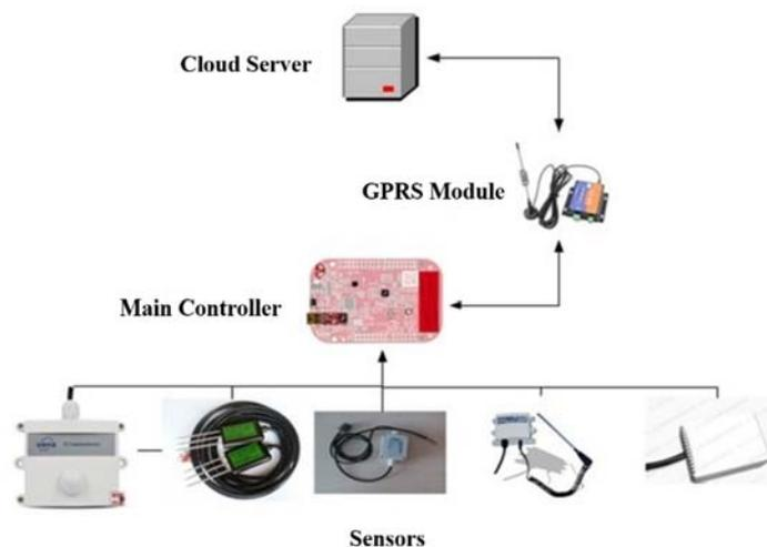
Fig.2 The hardware system architecture diagram
