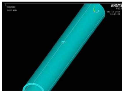
Fig.3 Three dimensional FEA structural model for pipeline
