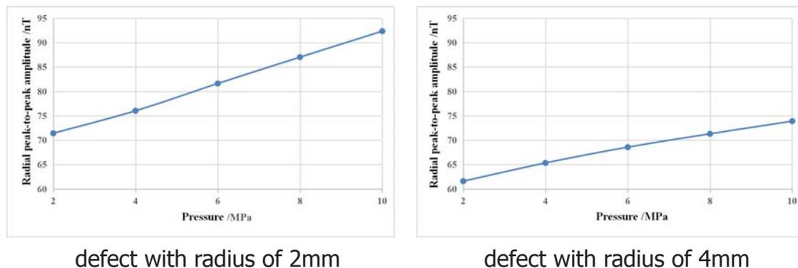
Fig. 6 An increase in the defect SMFL amplitude with increasing pipeline pressure
