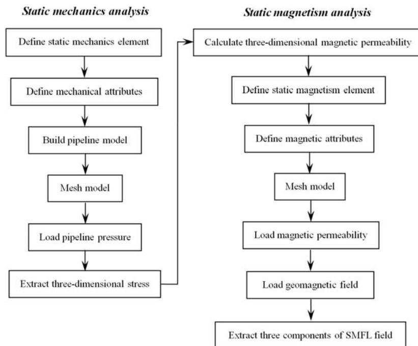
Fig. 2 Magneto-mechanical coupling scheme for pipeline magnetic testing
