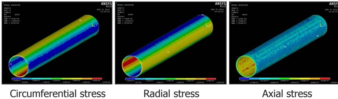
Fig. 4 Color contour plots of the pipeline stress field
