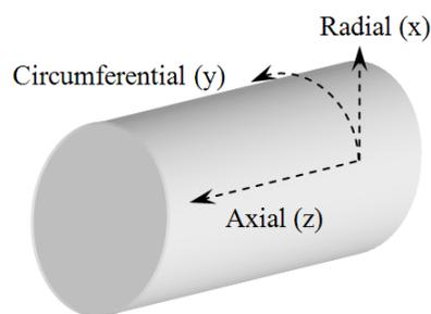
Fig. 1 Tridimensional pipeline cylindrical coordinate system
