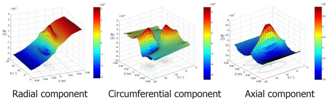
Fig.5 Surface mesh plots of the SMFL field components
