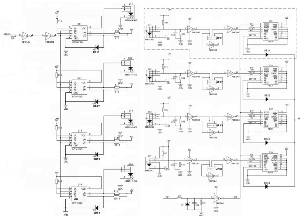
A. Fault signal sending board      B. Fault signal latch board
