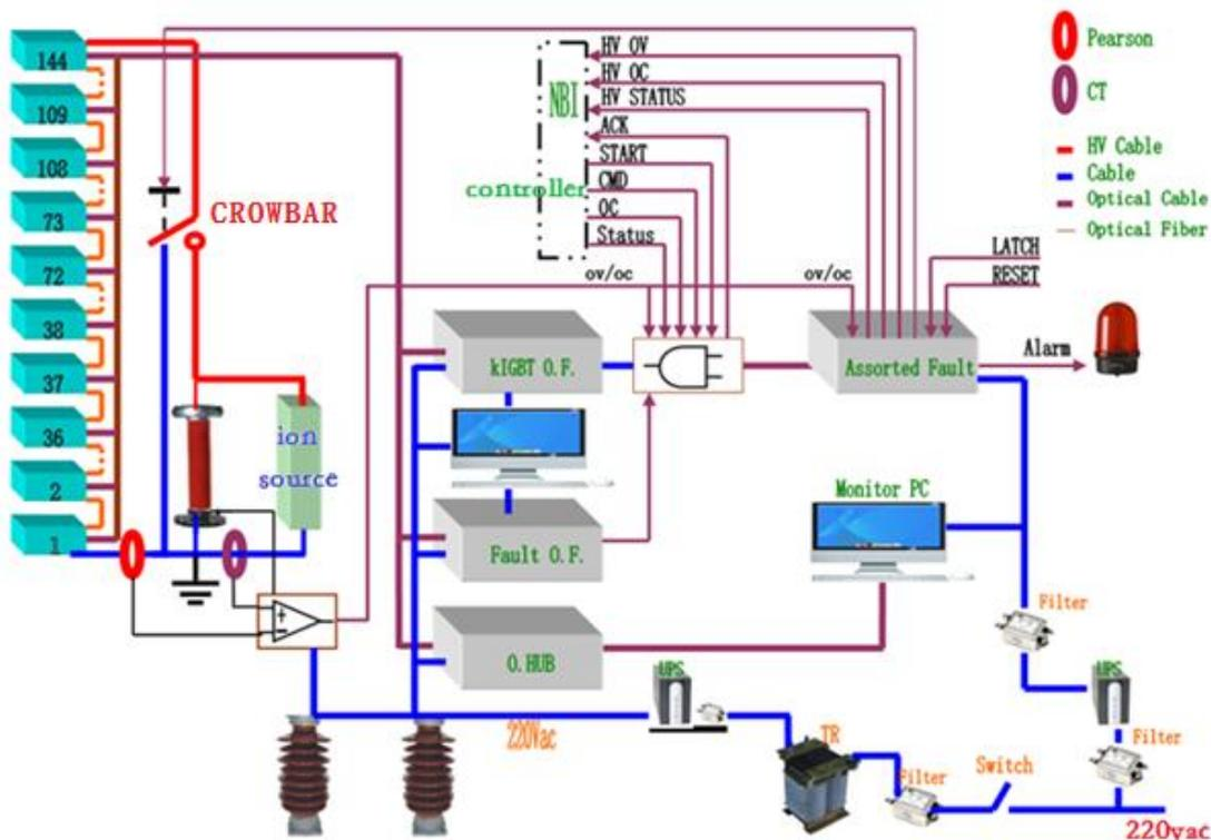
Fig.2 Chain protection control system block diagram
