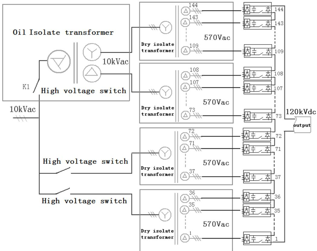
Fig.1 High voltage power supply topology
