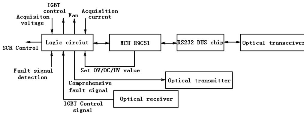
Fig.3 The principle diagram of the power supply module internal intelligent controller
