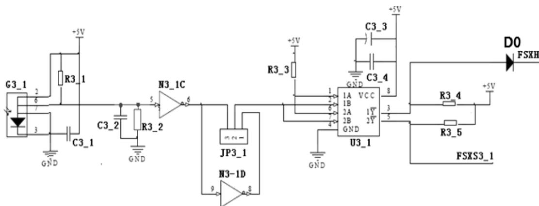
B. Light blockade signal circuit diagram
