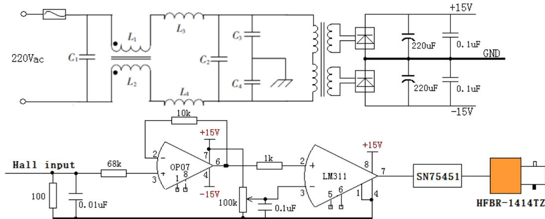
Fig.6 Over-current detection circuit
