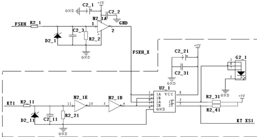
A. Light drive signal circuit diagram
