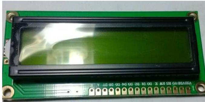
Figure 8 Physical figure of LCD1602 LCD module
