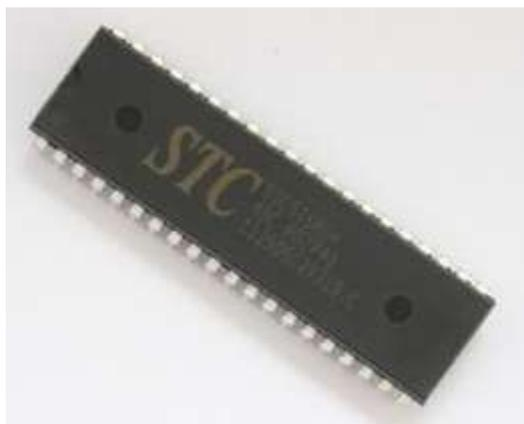
Figure 1 STC89C51 single chip microcomputer
