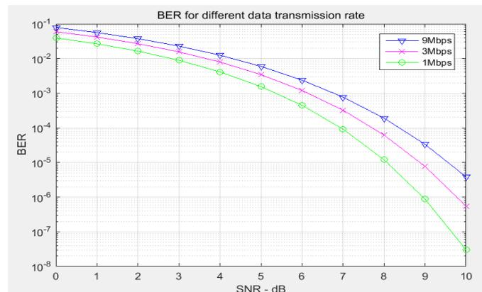
Figure 3: Signal-to-noise ratio and bit error rate of 16QAM-OW signals at different transmission rates
