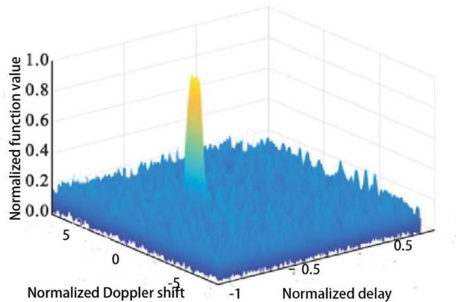
Figure 2: QAM-OW integrated signal fuzzy function
