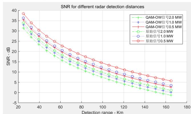
Figure 4: Probing distance and signal-to-noise ratio
