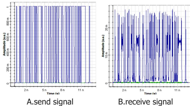
Fig 3.2 electric signal time domain waveform
