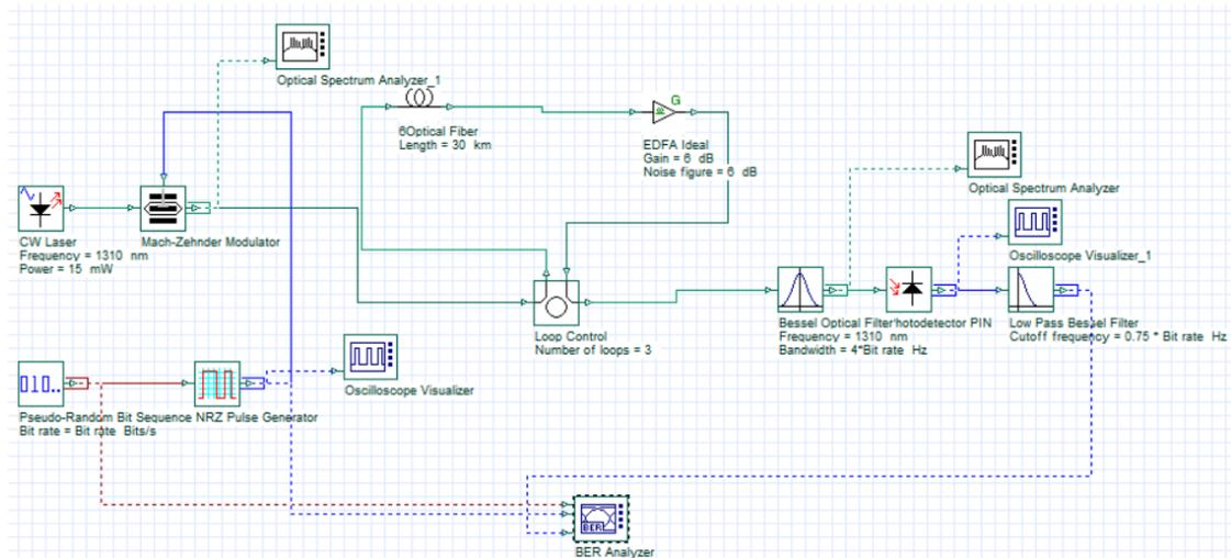
Fig 3.1 Optical fiber communication system diagram
