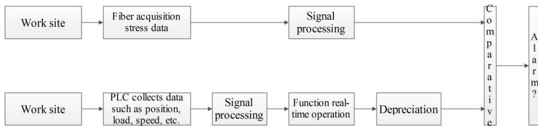
Fig.2 Alarm Execution Process
