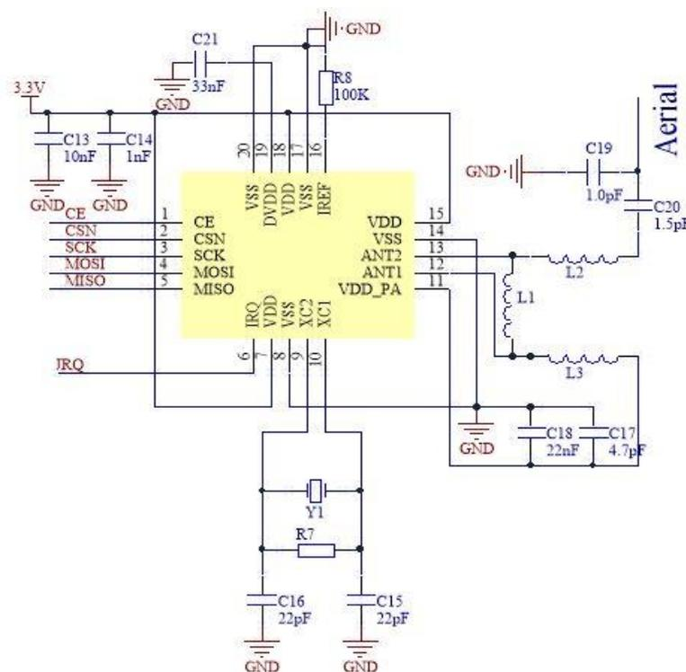
Figure5. The circuit of wireless communication module
