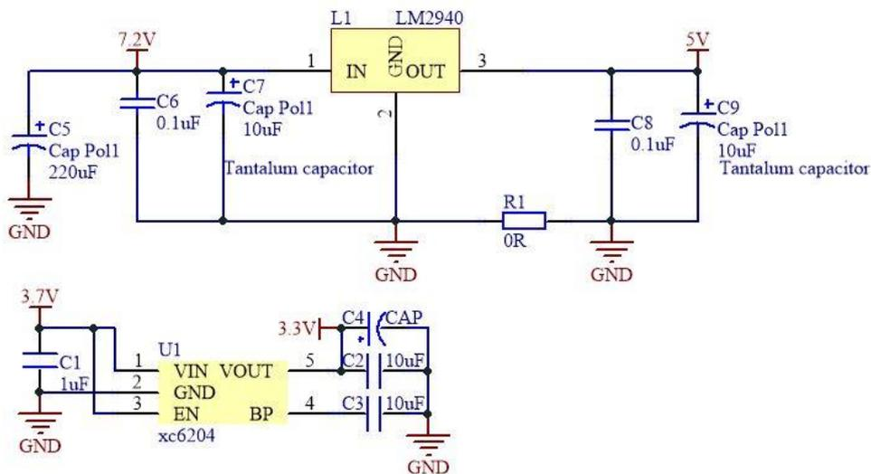
Figure3. The circuit of power management module
