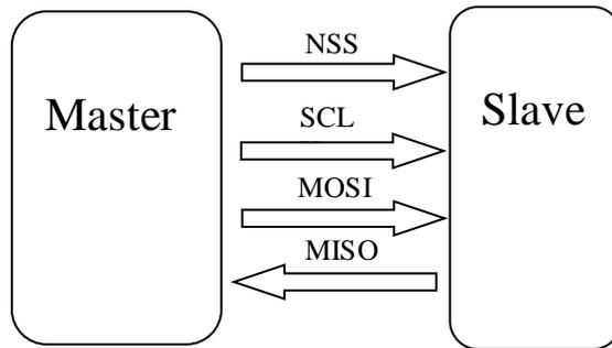
Figure 8. The protocol of wireless communication
