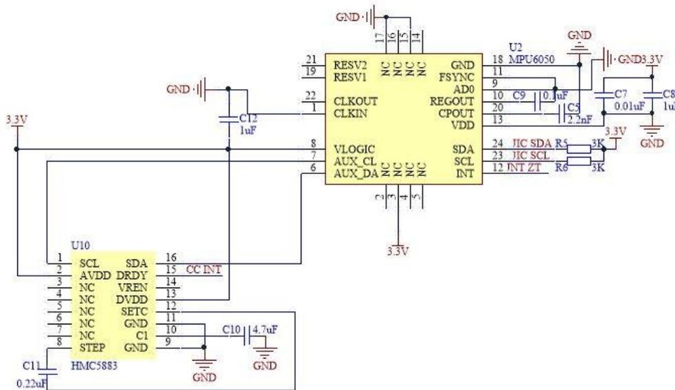
Figure 4. The Circuit of Attitude Acquisition Module
