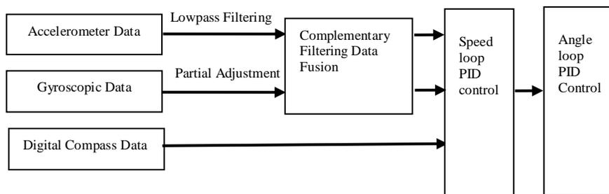
Figure 7. The flow of attitude algorithm
