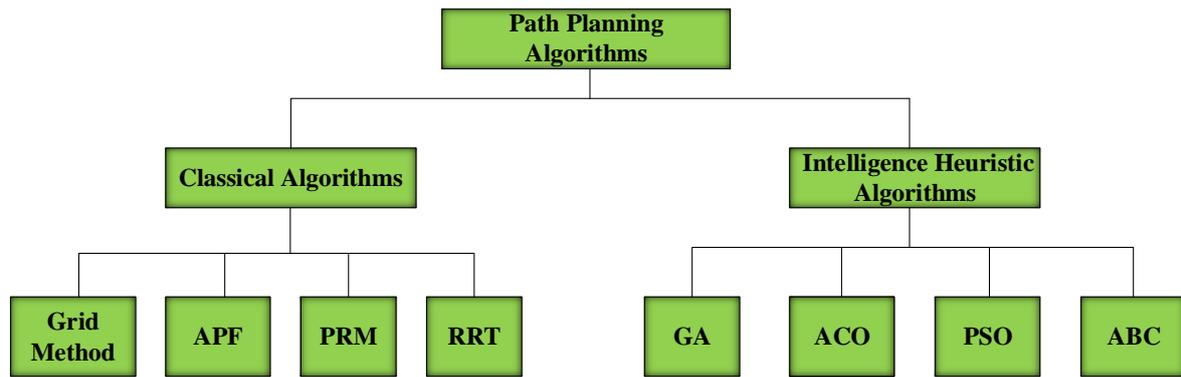
Fig 1. The classification of robot path planning algorithms
