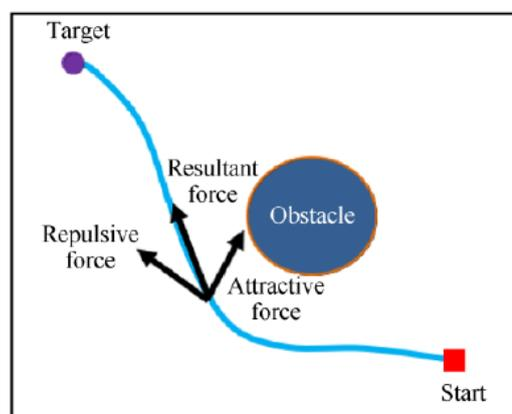
Fig3. Mobile robot navigation by APF approach
