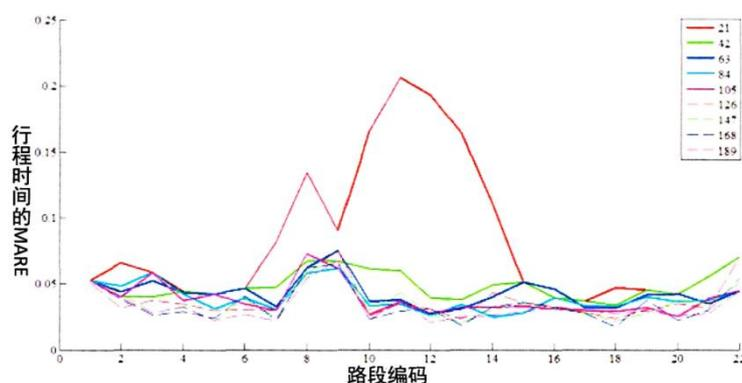
Figure 3 Average absolute relative error MARE of travel time under different layout schemes
