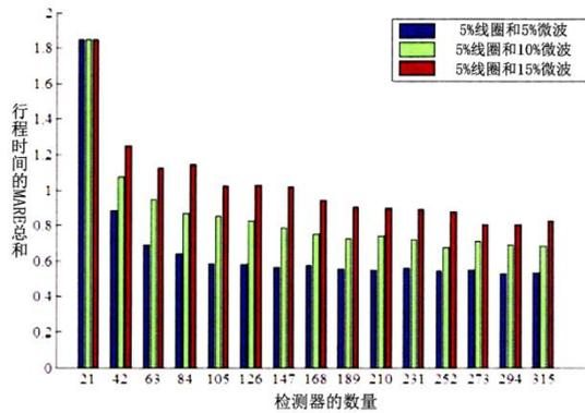
Figure 1 Comparison of Detector Layout Schemes under Different Detection Accuracy
