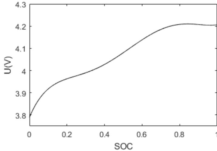
Fig. 5 SOC and  $U$  relationship diagram
