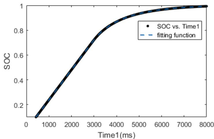
Fig. 4 SOC and t relationship diagram
