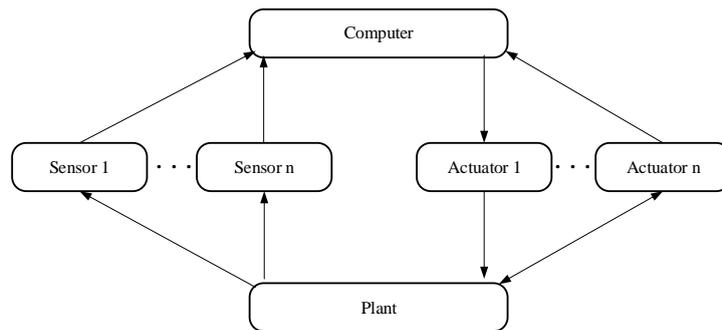
Fig. 1 Structure of Distributed Control System
