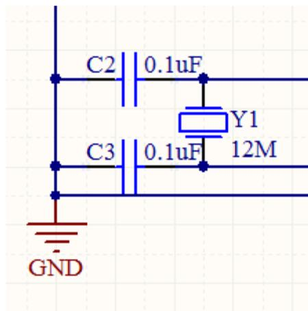
Fig. 6 Oscillation circuit inside the microcontroller
