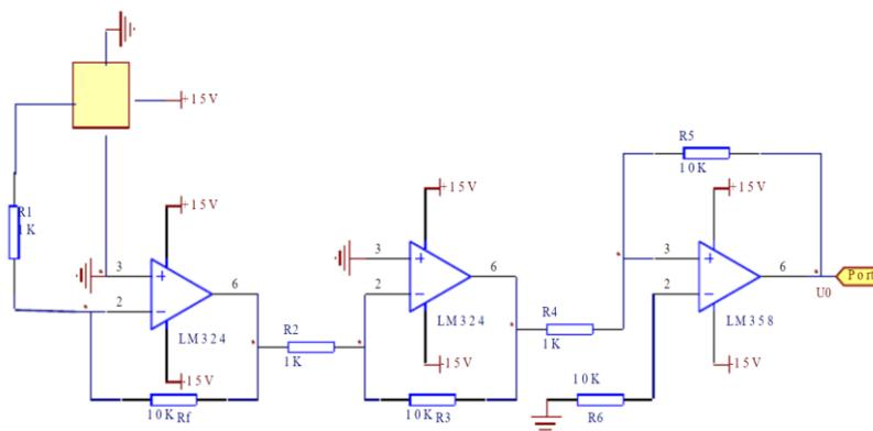
Fig. 4 Signal preprocessing circuit
