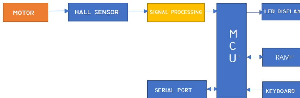
Fig. 1 Overall hardware design
