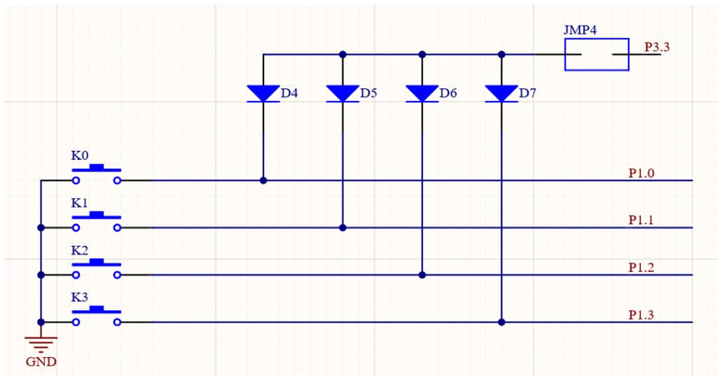
Fig. 6 Button circuit
