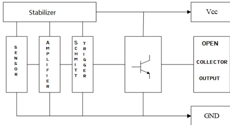
Fig. 2 The internal structure block diagram of the Hall sensor
