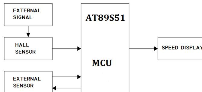
Fig. 3 The principle block diagram of the MCU and Hall sensor system
