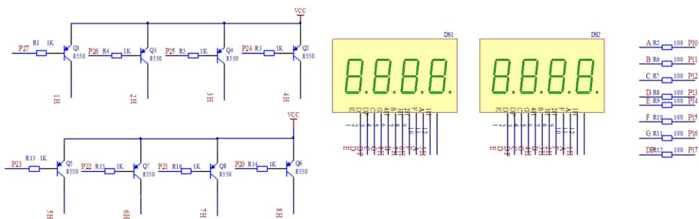
Fig. 5 Digital tube display circuit
