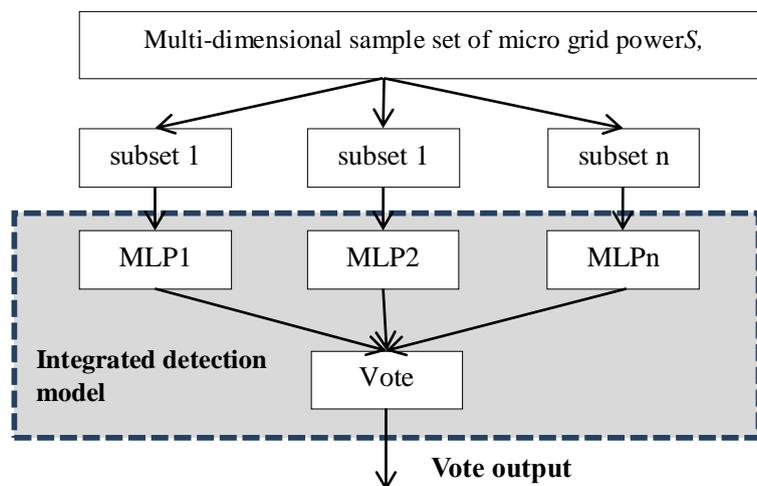
Fig 2. Structure of the integrated classifier
