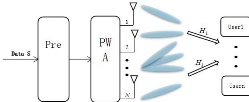
Figure 1 Multi-channel communication system model
