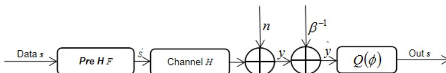
Figure 2 Principle diagram of ZF precoding algorithm
