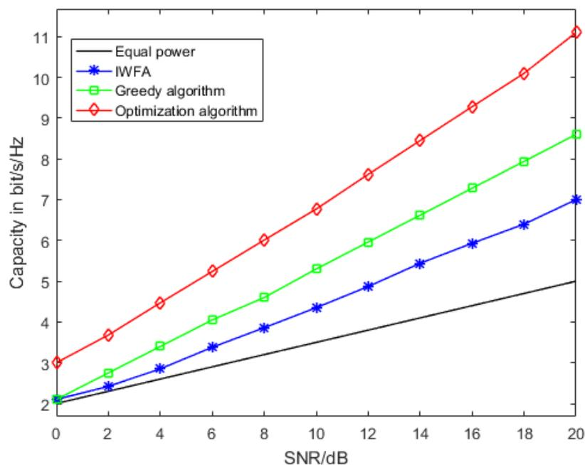
Figure 4 Spectrum efficiency under different algorithms
