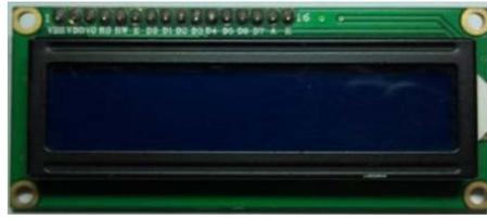
Figure 6 LCD1602 LCD module
