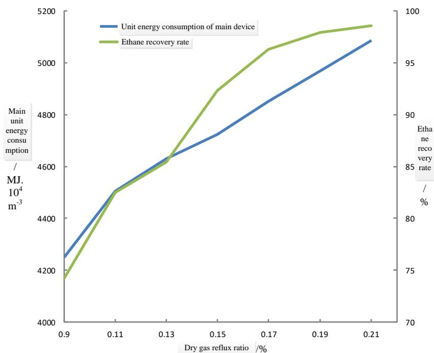
Fig. 2 The change curve of unit energy consumption and ethane yield and reflux ratio of external dry gas
