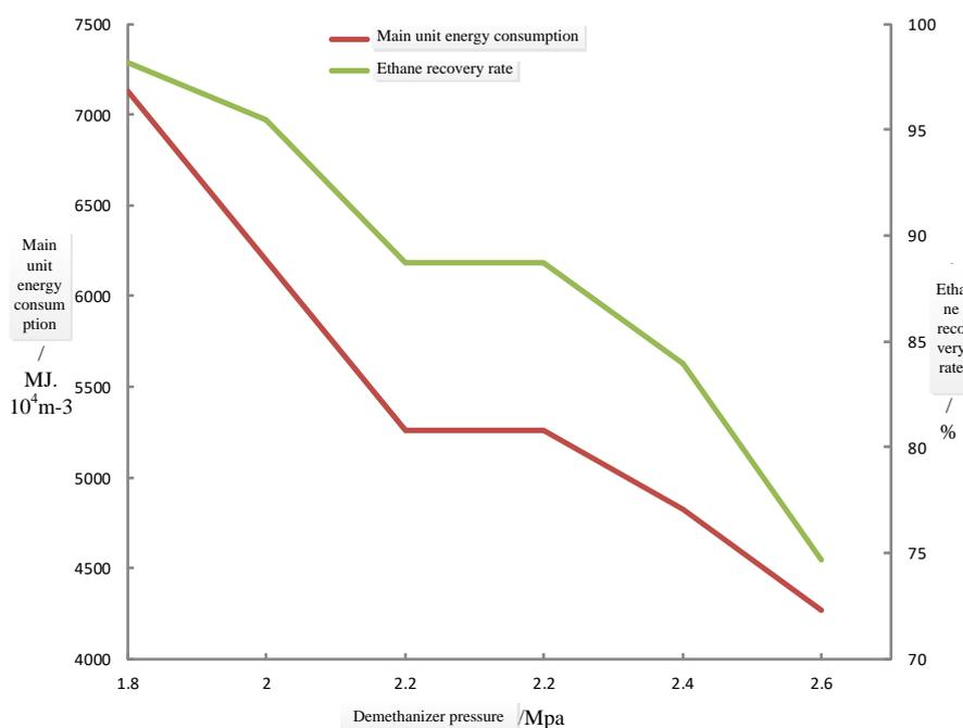
Fig. 3 The change curve of unit energy consumption and ethane yield and pressure of demethanizer
