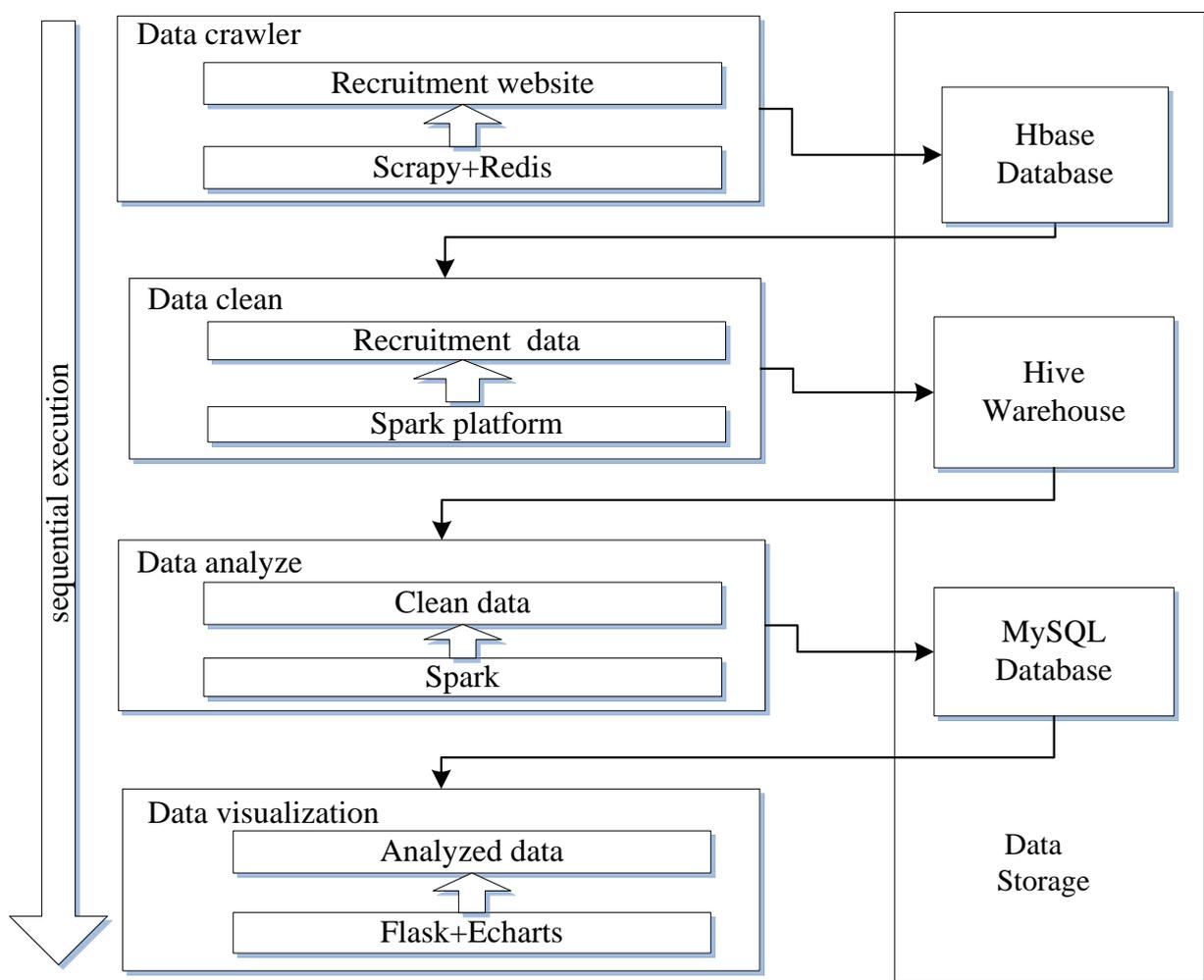
Fig. 1 The system architecture of IoT talent analysis platform
