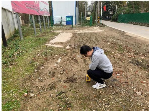
Figure .2 Portable XRF instrument(Sciaps) and on-site detection
