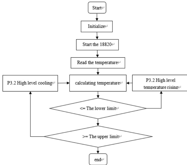
Figure 6 Temperature control flow chart
