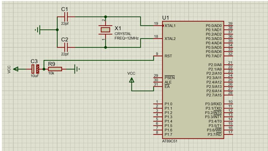
Figure 4 Minimum system diagram of MCU
