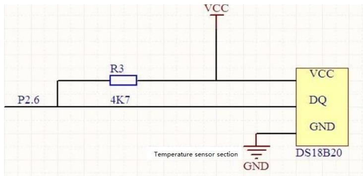
Figure 5 Schematic diagram of temperature sensor
