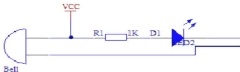
Figure 9 Alarm circuit diagram
